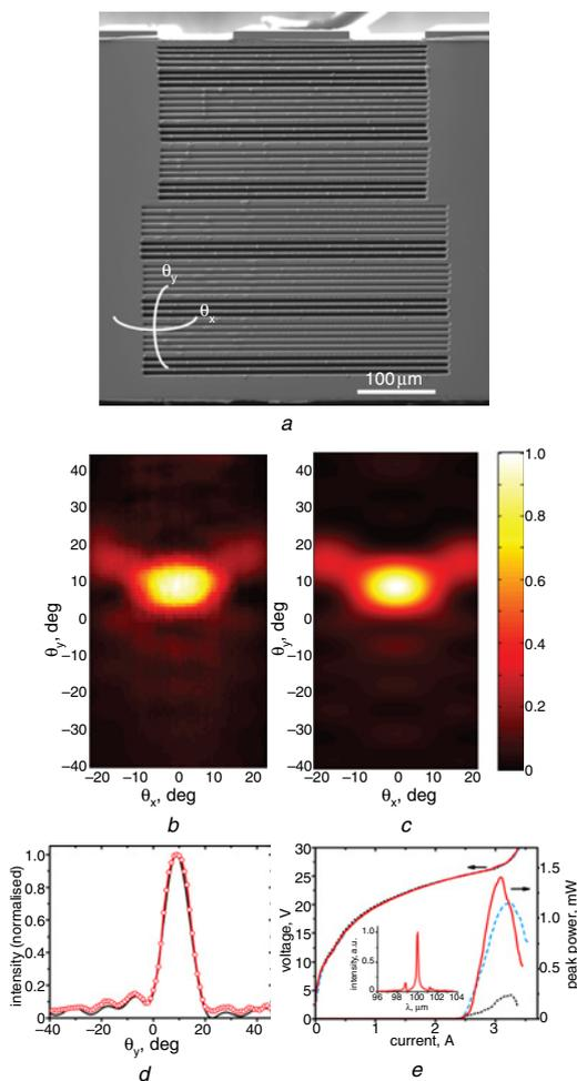
**Fig. 7** Experimental results for  $\lambda_0 = 100 \mu\text{m}$  QCL with metasurface-based collimator
