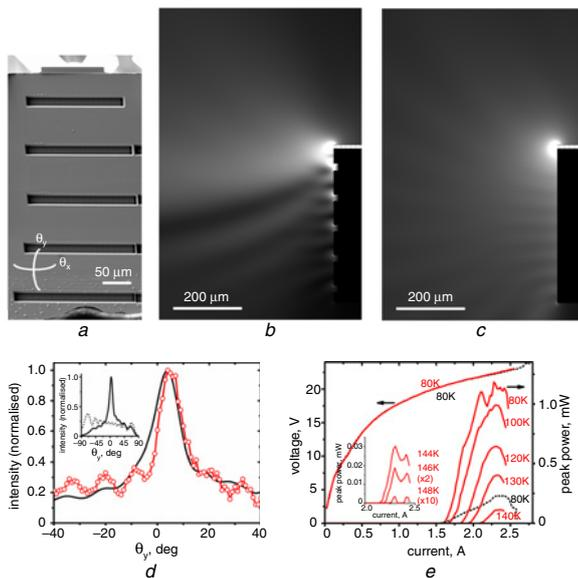
**Fig. 3** Results for  $\lambda_0 = 100 \mu\text{m}$  THz QCL with second-order-grating collimator directly sculpted into GaAs facet
