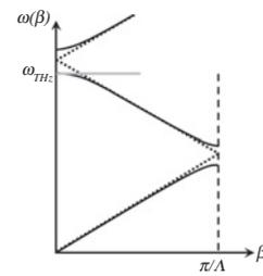
**Fig. 1** Schematic dispersion curve of SPPs on metallic surface sculpted with second-order grating (solid line)
