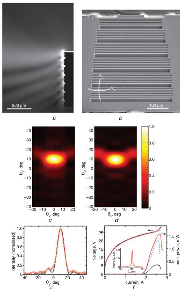
**Fig. 5** Simulation and experimental results for collimator consisting of second-order grating and spoof SPP structures
