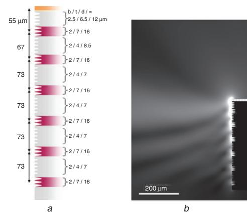
**Fig. 6** Design and simulation for metasurface-based collimator
