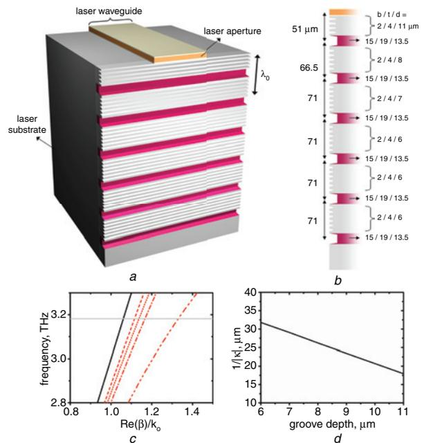
**Fig. 4** Design of collimator consisting of second-order grating and spoof SPP grooves
