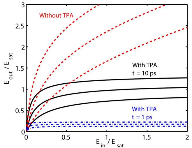
Fig. 1. (Color online)  $E_{\text{out}}$  versus  $E_{\text{in}}$  curves without TPA (dashed curve) and with TPA assuming FWHM pulse widths of 10 ps (solid curve) and 1 ps (dotted-dashed curve). The SOA parameters are given in the text and correspond to the InGaAsP SOA in [3].  $E_{\text{sat}} = 100 \text{ pJ}$ . In each case, the three curves correspond to unsaturated material gain values ( $g_o$ ) of 800, 1200, and  $1600 \text{ cm}^{-1}$ .
