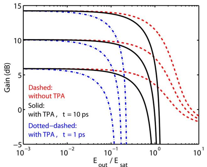
Fig. 2. (Color online) SOA gain without TPA (dashed curves) and with TPA assuming FWHM pulse widths of 10 ps (solid curves) and 1 ps (dotted-dashed curves). The SOA parameters are given in the text and correspond to the InGaAsP SOA in [3].  $E_{\text{sat}} = 100 \text{ pJ}$ . In each case, the three curves correspond to unsaturated material gain values ( $g_o$ ) of 800, 1200, and  $1600 \text{ cm}^{-1}$ .
