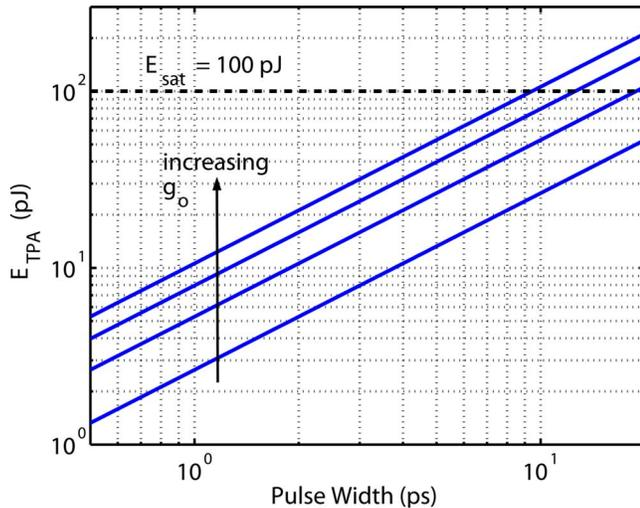
Fig. 3. (Color online) Values of  $E_{\text{TPA}}$  are plotted as a function of the FWHM pulse width  $\tau$ . The SOA parameters are the same as in Figs. 1 and 2. The four curves correspond to unsaturated material gain values ( $g_o$ ) of 400, 800, 1200, and 1600  $\text{cm}^{-1}$ .
